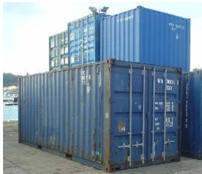
Figure I.4. A twenty-foot container (1 TEU).
