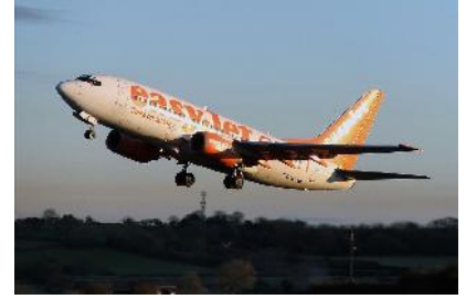
Figure C.11. Boeing 737-700: 30 kWh per 100 passenger-km. Photograph © Tom Collins.
