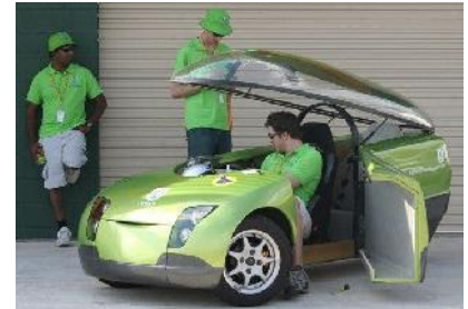
Figure 20.42. The TREV. 6 kWh per 100 km . Photo from www.unisa.edu.au .
