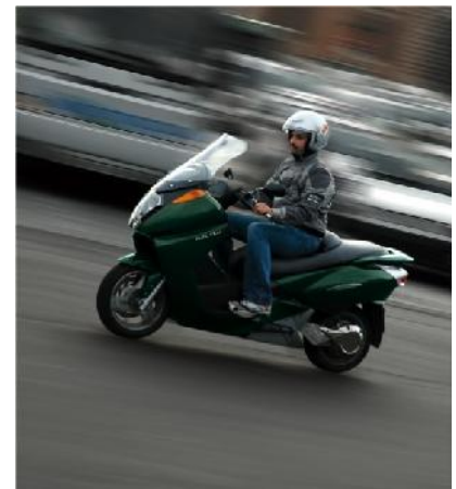
Figure 20.44. Vectrix: 2.75 kWh per 100 km . Photo from www.vectrix.com .
